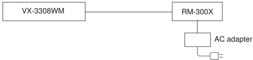
When supplying power to the RM-300X from the optional AD-246 AC Adapter using an STP category 5 straight cable or over 4-pair shielded CPEV cable, the maximum length of connection cable (excluding power line) is 1200 m regardless of the type of cable and the number of remote microphone extension units.
